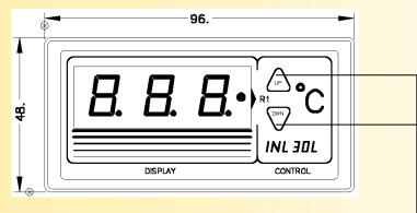
A ponctual push on one of these two keys allows to displays the alarm threshold. When the threshold value is displayed a prolonged push on the "up" key or on the "down" key allows to increment or decrement the alarm threshold. If the keys aren't pressed during few second, the adjustment is automatically validated and the device switch in measure mode.
